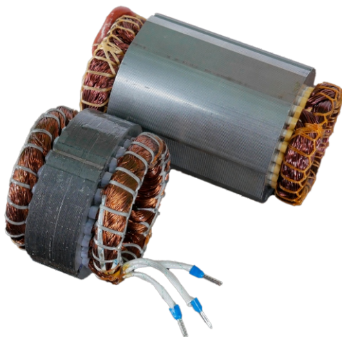
Comparing the stator dimensions of a "Sovelmash" mitre saw with the stator of a standard winding motor
