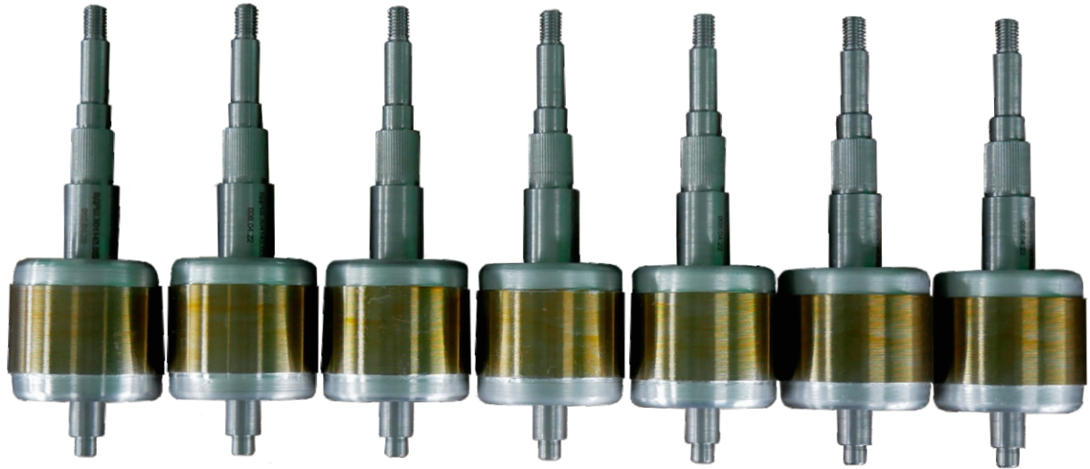
Rotors for a universal built-in drive designed by "Sovelmash"
