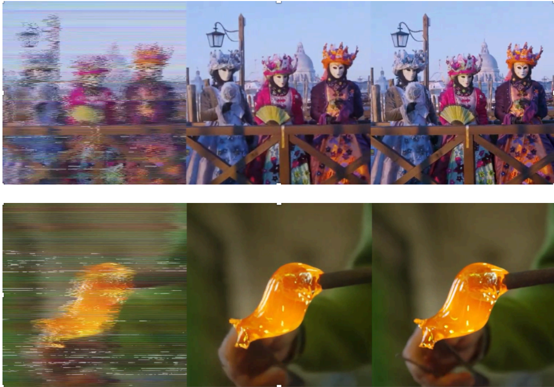
Fig. 11 - examples of video frames restoration: left) input: degraded frames; middle) output of the network; right) ideal result, i.e. original high quality frame used to produce the degraded version.
