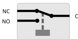
Relay configuration (not energised).
