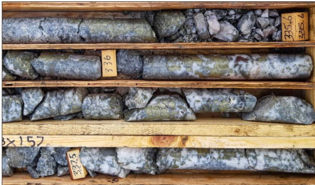
Plate 7.7 JT Deposit – Footwall Copper Zone (FWCZ) in Hole JT19-089 (20.7m @ 2.38% Cu, 31.8 g/t Ag, 4.86% Zn)
