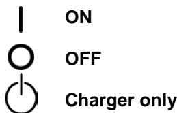
When switched to "on", the product is fully functional. The inverter will come into operation and the LED "inverter on" will light up.
