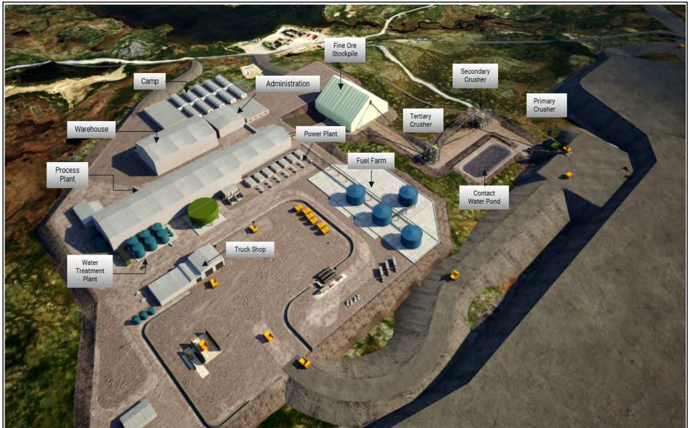
Figure 18-7: Overall On-site Infrastructure Layout
