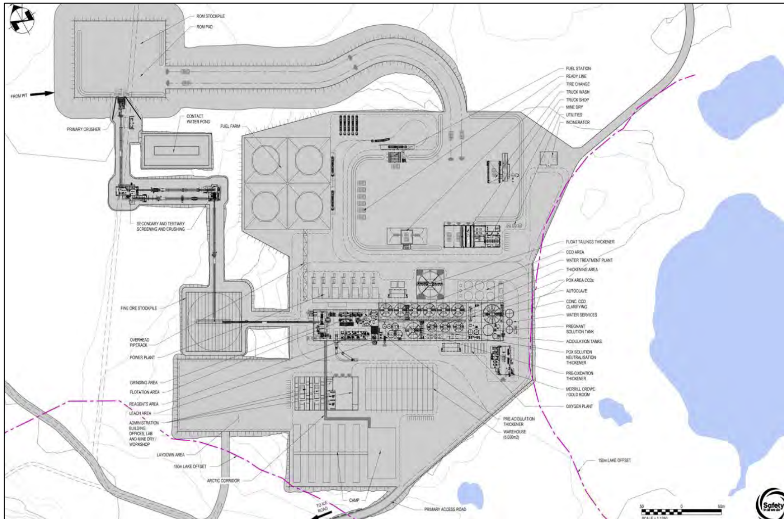
Figure 17-2: Overall Process Plant Layout
