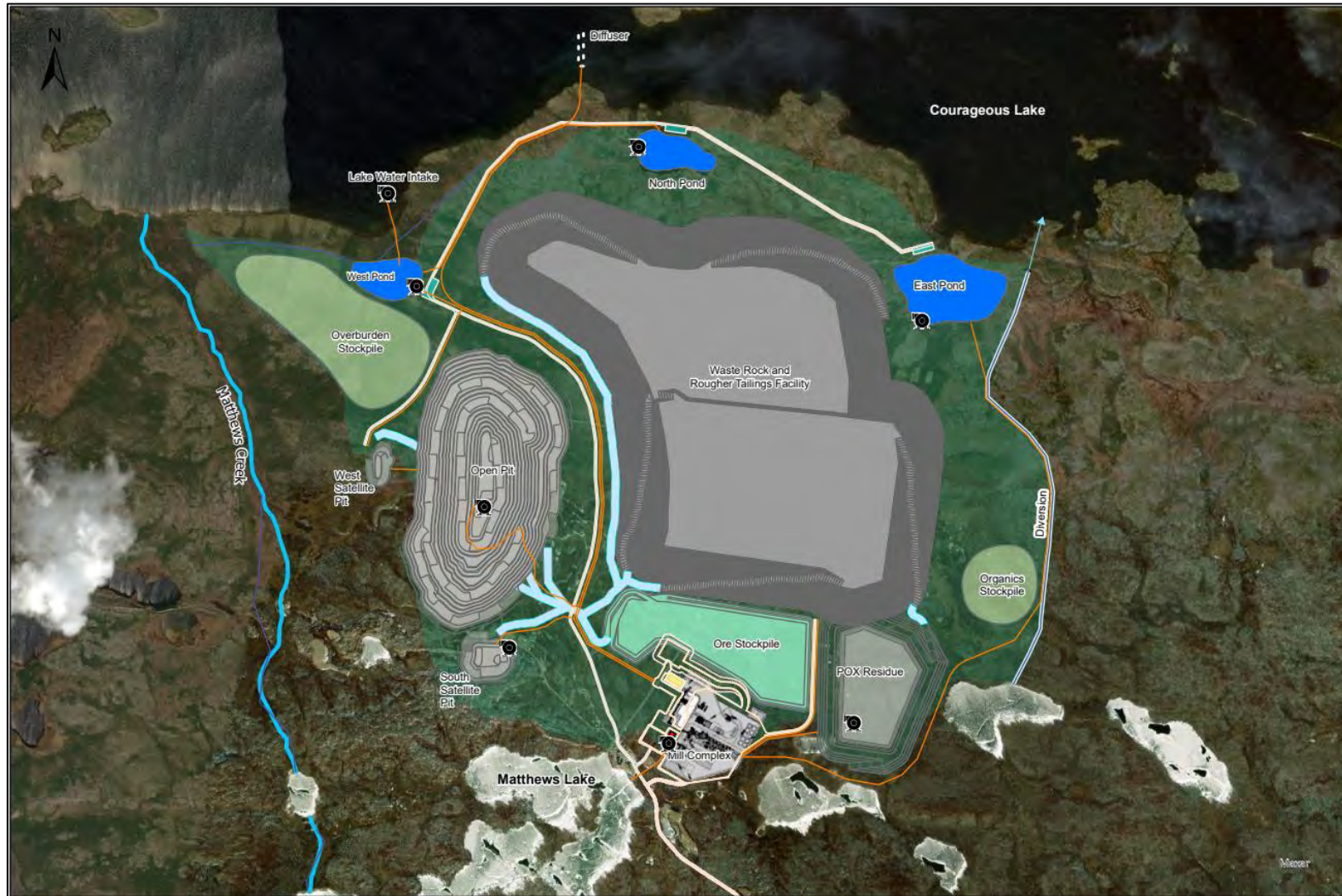
Figure 18-14: Water Management and Mine Infrastructure
