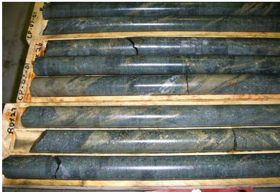
Figure 11b: Disseminated pyrite with stringer zone chalcopyrite in augen schist from drill hole CP-07-1
