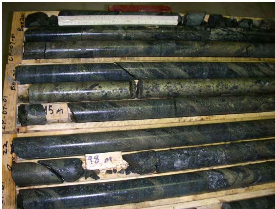
Figure 11a: Massive pyritic sulphide and chalcopyrite from drill hole CP07- 01
