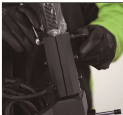
5. Tighten the screws and lock nut to secure the stem
