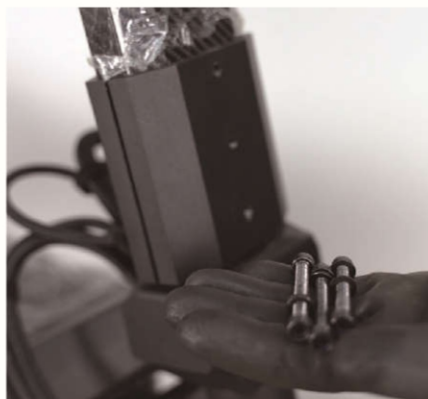
2. Use 3 sets of M6x60 long screws with M6 lock nuts and M6 washers
