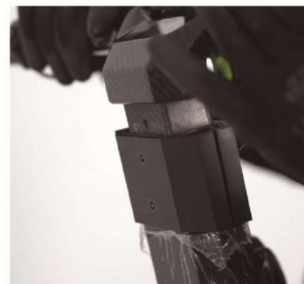
6. Slot the top stem adaptor into the top of the stem
