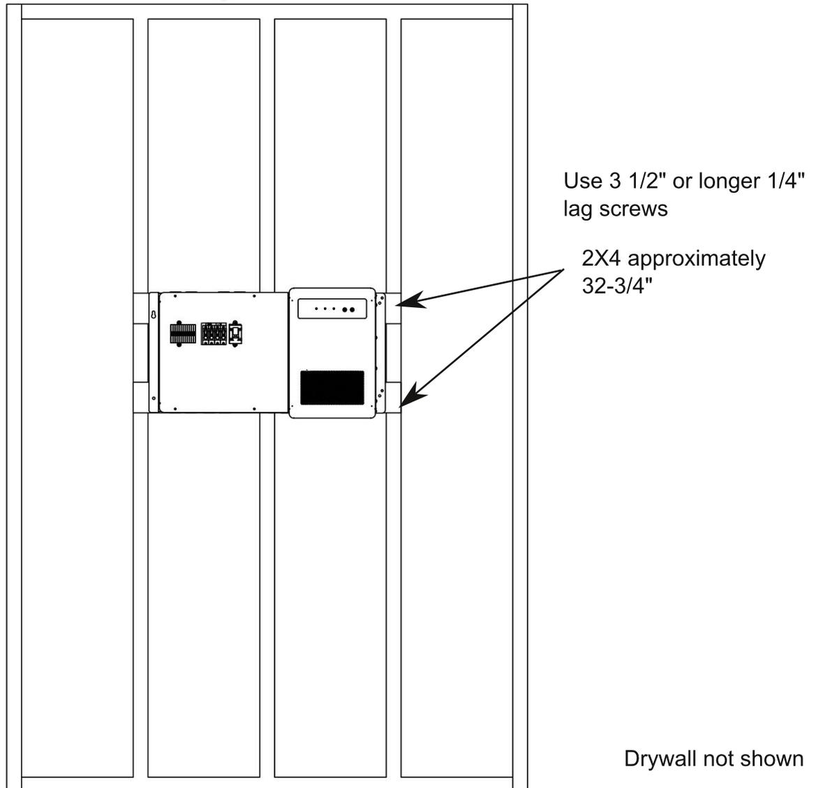
**Example:** Wall mounting the Conext SW E-Panel and Conext SW Inverter
