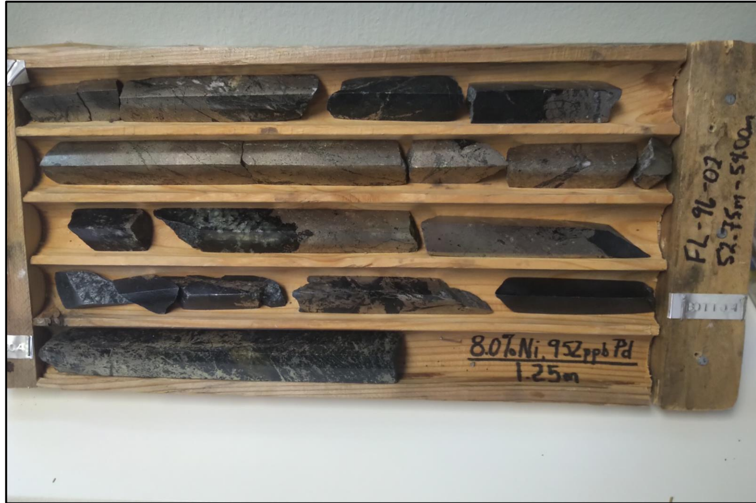
Quartered polished interval from Hole TFL-96-02 – 52.75m to 54.00m grading 8.0% nickel over 1.25m
