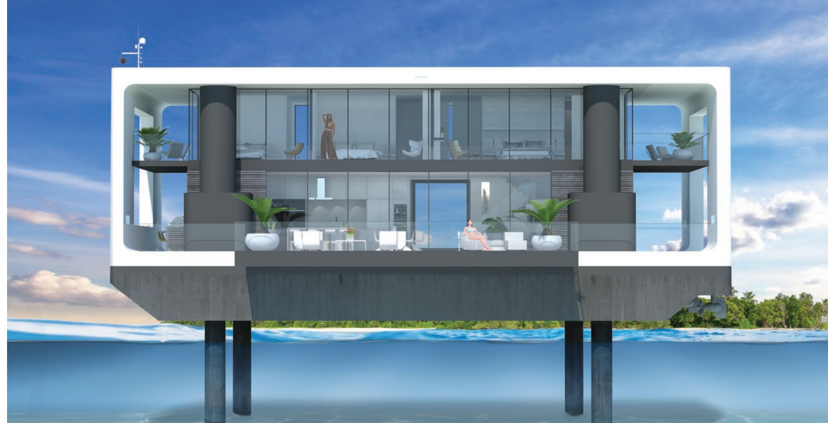
The hydraulic pilings raise the vessel above the waves
