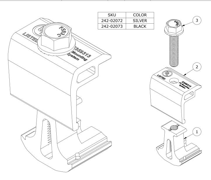
CLAMPS FIT 30-46MM THICK MODULE FRAMES
