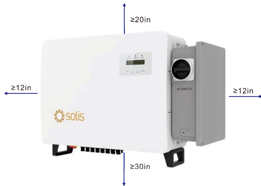
Figure 3.2 Clearance distances requirement for the inverter
