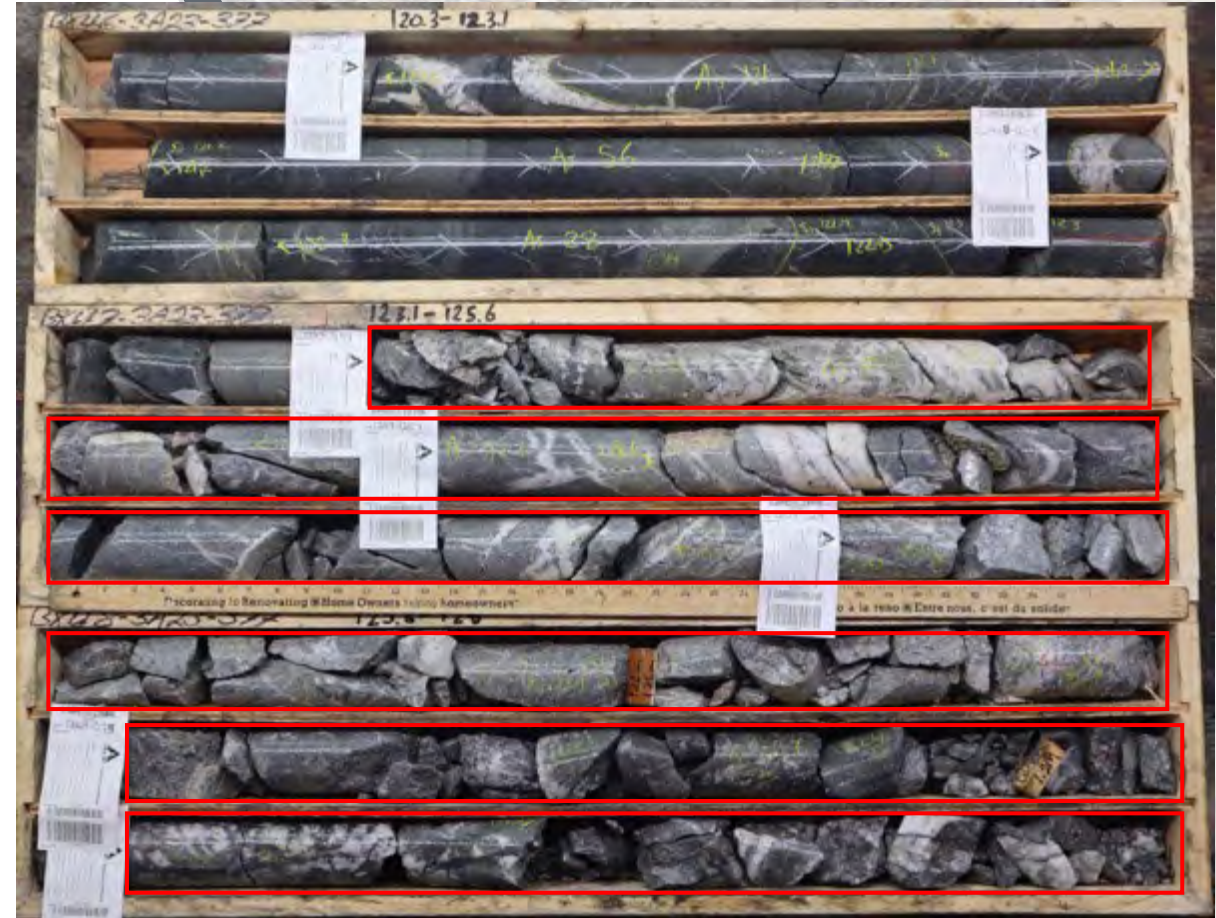
High-grade gold mineralization extending the Spades zone 250m SE (7.2m @ 7.6 g/t)
