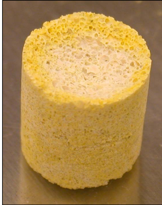
Figure 4. BeO structure after dissolution of uranium
