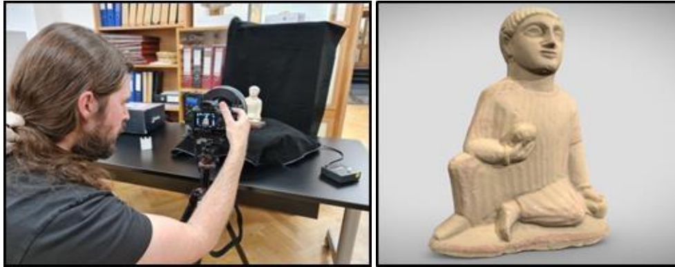
Figure 19 The process of Photogrammetry was used to carefully digitize the artifacts to be used in the video game. On the right, one of the reconstructed models, “Temple Boy - Cypriot Sculpture 4th century B.C.” is shown. The model can be interactively viewed at: https://skfb.ly/oDN7X .
