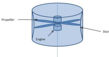
Lift engines are ducted fans each one composed by:
