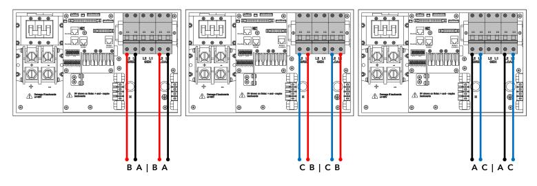
Figure 38: Example of correct phase sequence
