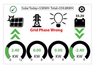
Figure 37: Grid phase wrong error
