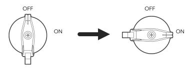
Figure 20: Built-in PV DC disconnect
