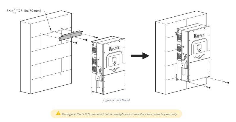
H. Mount the inverter in the optimal orientation as shown below.
