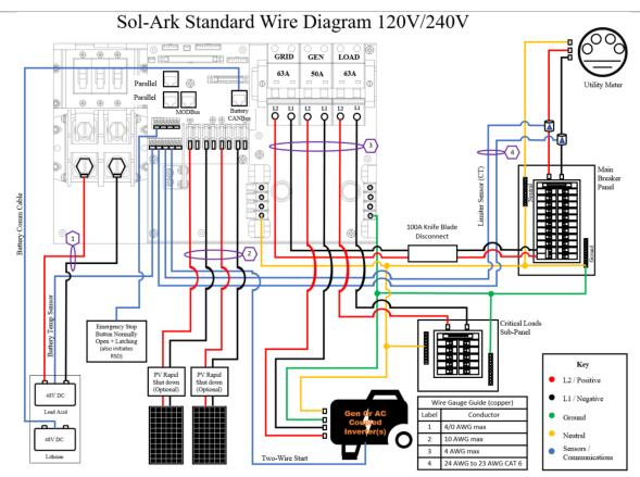
NOTE: Location of the neutral-to-ground bond will depend on local code NOTE: Size of disconnect will depend on required passthrough
