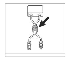
a) Installation of small suppressor on appliance power cord
