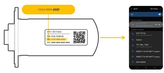
Figure 41: E4A0-##### serial number and EAP network
