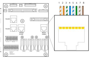
Figure 34: RJ-45 port configuration
