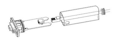
Figure 39: Connecting Wi-Fi dongle to ethernet
