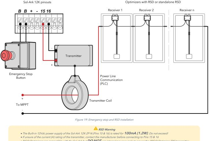
• TIGO Optimizers are compatible with the Sol-Ark but DO NOT use internal power supply to power the "TIGO Optimizer TX" transmitter
