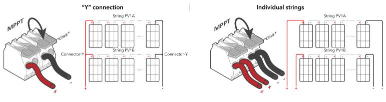
Figure 9: MPPT wiring and PV connections
