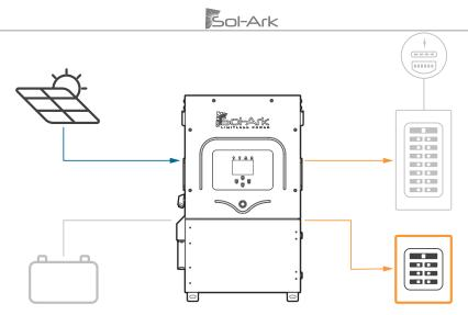
Figure 30: Limited Power to Load + Grid Sell
