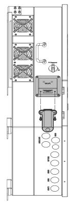
Figure 40: Connecting Wi-Fi dongle to Sol-Ark 12K-2P-N
