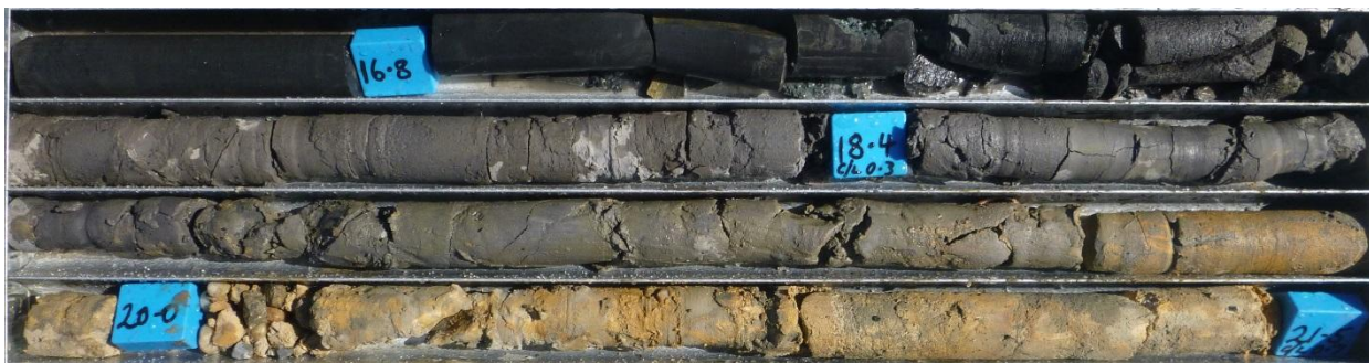
Plate 8 – Characteristic transition from pristine basalt (black) to extremely weathered and smectitic remnant basalt and clay (grey) to an arkose sandstone (orange-brown). Hole CCD15-01.
