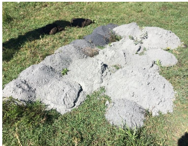
Plate 6 – QCP15-04 hole cuttings showing clay fines at depth
