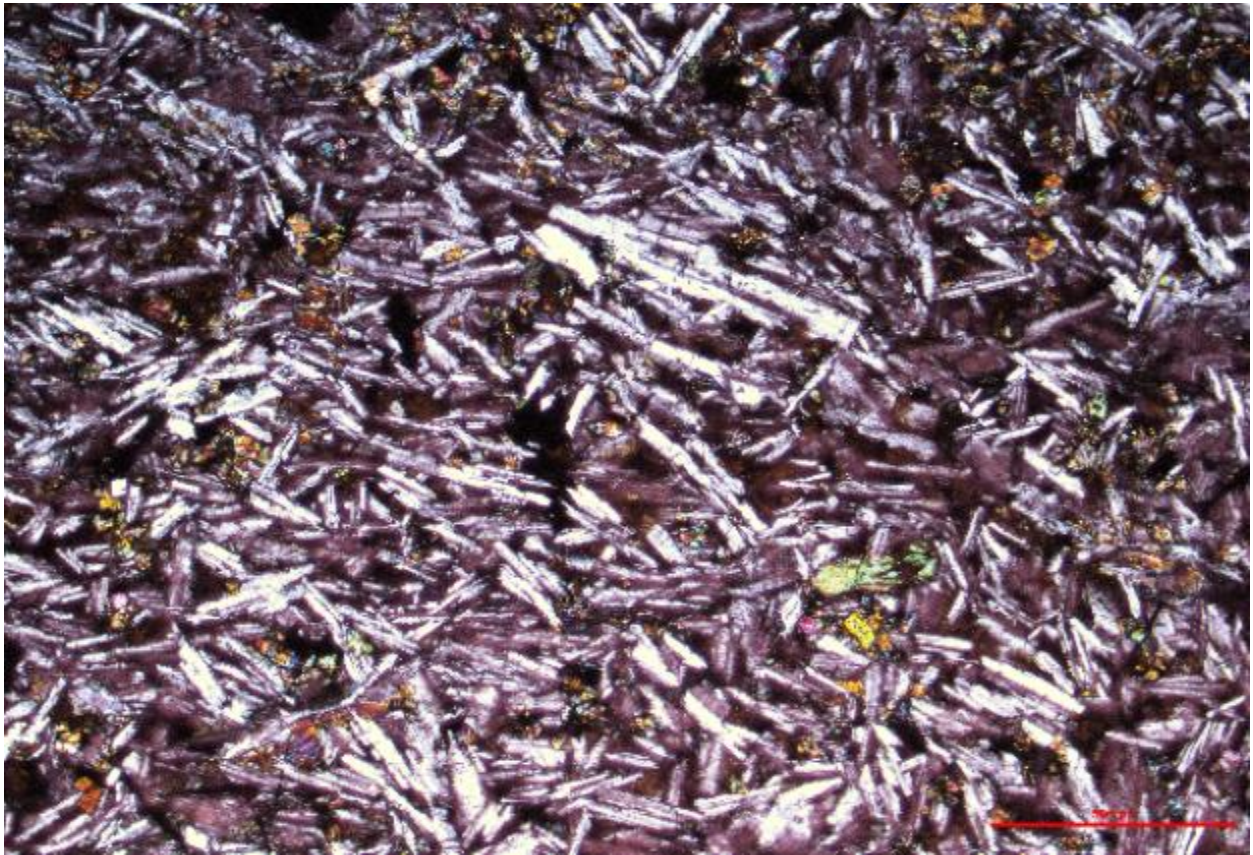
Plate 2. Microphotograph displaying representative mineral assemblage of the basalt including abundant plagioclase laths, pyroxene and olivine with opaques and semi-opaque volcanic glass.
