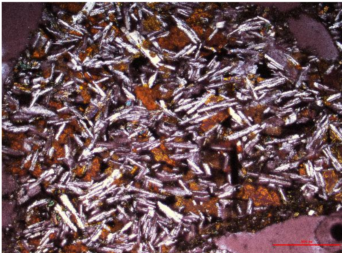
Plate 2. Microphotograph displaying a basalt fragment which exhibits comprehensive devitrification as bright orange interstitial replacement resulting in smectite clays and minor chlorite. Image shown in cross polarised light.
