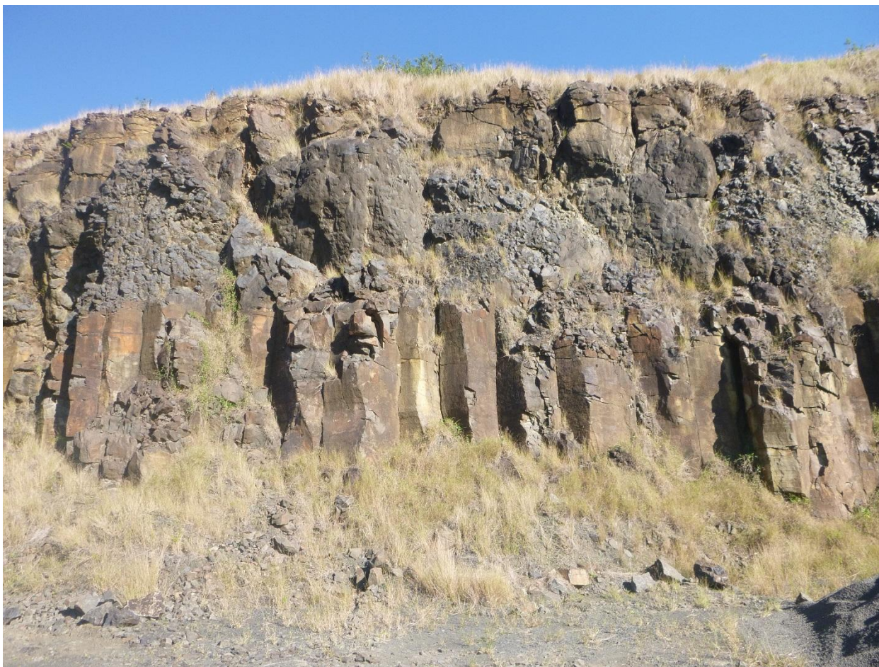
Plate 7 – Photograph of the adjoining quarry's western face displaying the full profile of the basalt including superficial soils and eluvium, agglomerate basalt and columnar basalt at depth.
