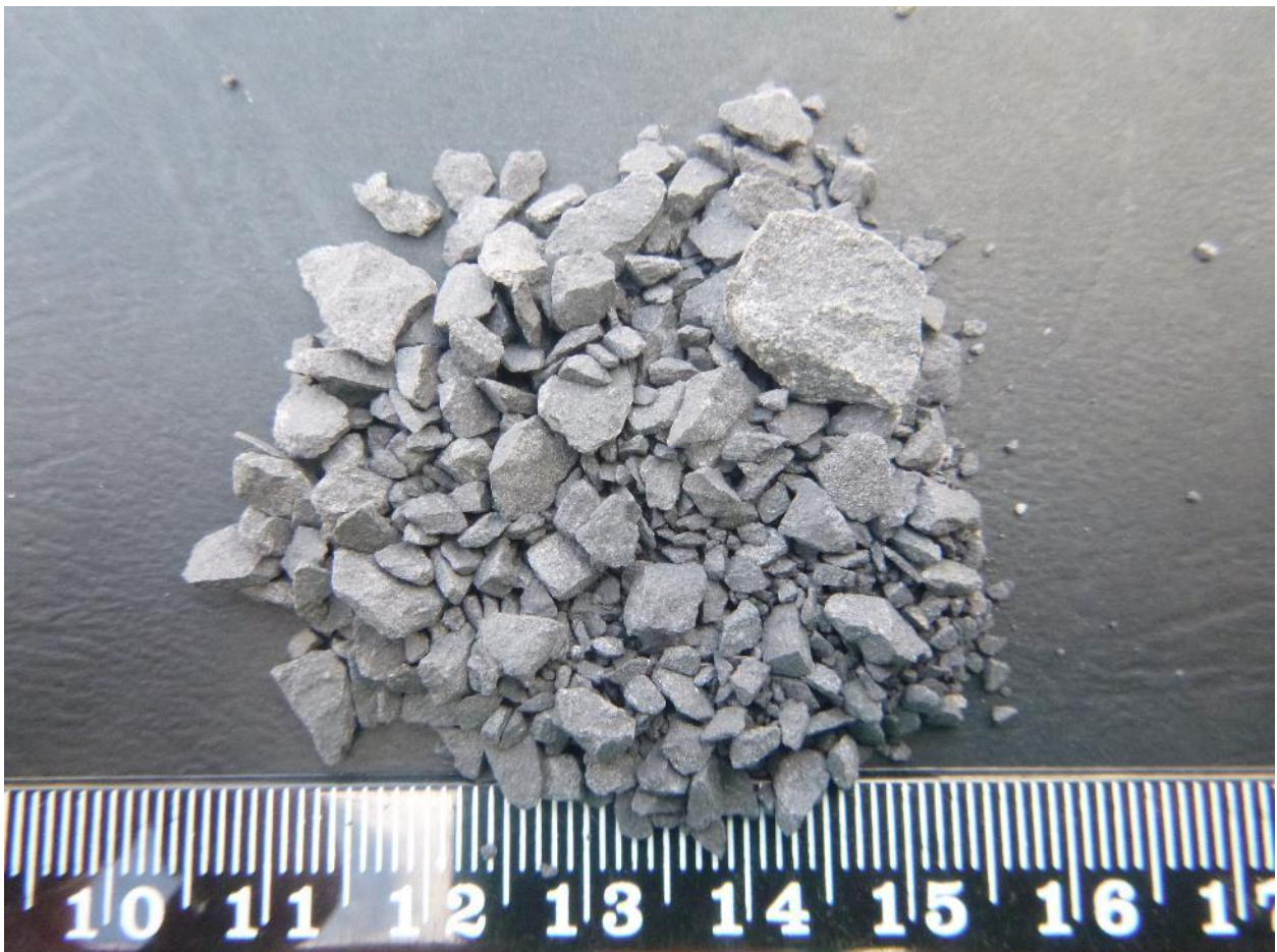
Plate 1. Photograph displaying unweathered basalt composed of fine plagioclase in a mafic groundmass including pyroxene and ferro-magnesian glass. Residual dust is minimal with fractured faces containing little stubborn clay fines.
