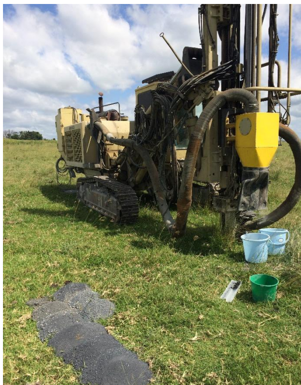
Plate 1 – Atlas Copco ECM660 Percussion Drill Rig
