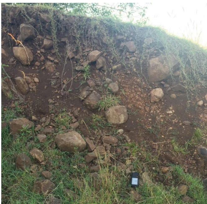
Plate 2 – Soil and Eluvium Profile within Dozer Cut Showing Basalt Floats
