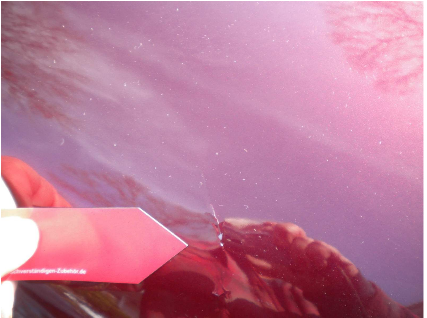
crack in work of hood
