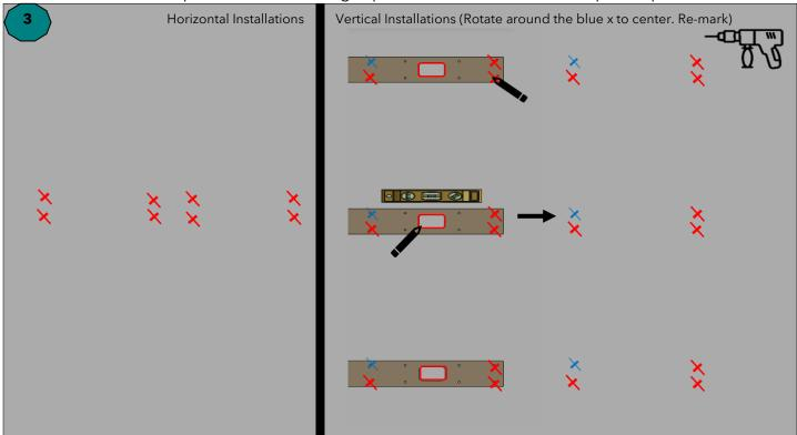
**4.** Affix the larger mounting bracket into the wall. Make sure that both wall brackets are leveled. Screw in the security screw into the center mounting location using the included hex key. Leave 1/5" inch of room when tightening.
