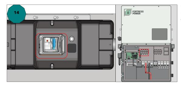
**14.** Turn On the DC Battery Breaker and Hybrid inverter DC Battery Breaker.
