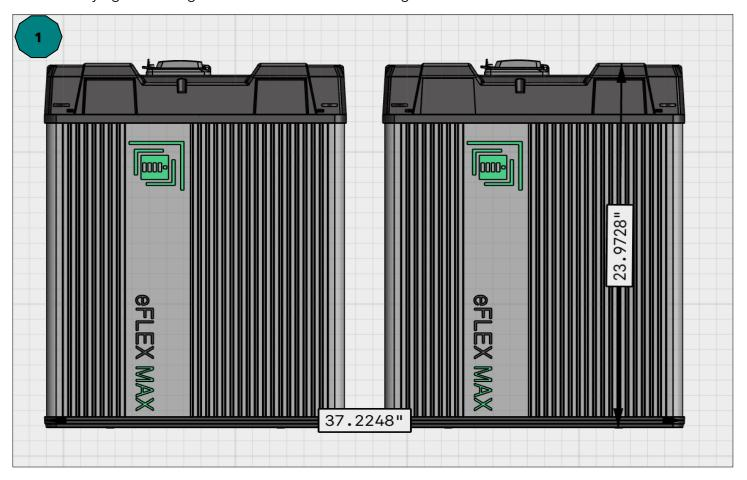
2. Use provided wall mounting template to mark out wall mount position.
