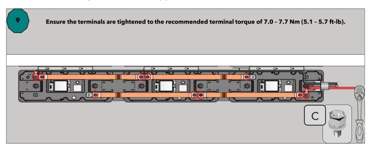
CAUTION! Installation should be designed to minimize the voltage drop between batteries. There are a few best practices: Maintain identical wire length and wire construction from each Fortress Power Battery terminal to the common bus. If Charge and discharge current exceeds 250amps a battery combiner/bus bar is required.
