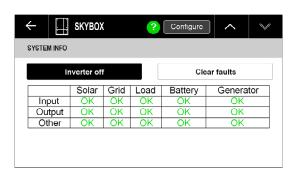
Most faults are automatically recoverable. The only faults that remain active under *Inverter Fault Status* are those that could not be handled automatically and need to be manually cleared.
