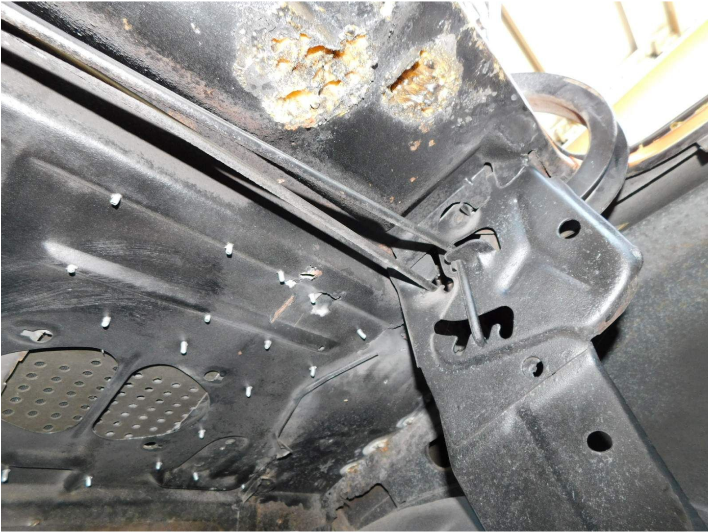
Package tray underside (rust repair)
