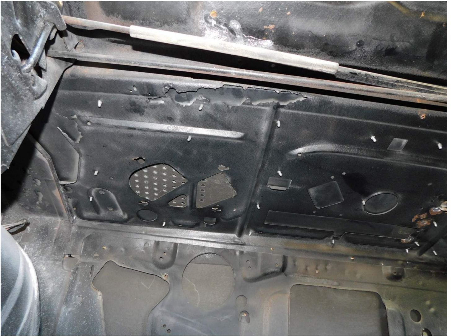
Package tray underside (rust repair)
