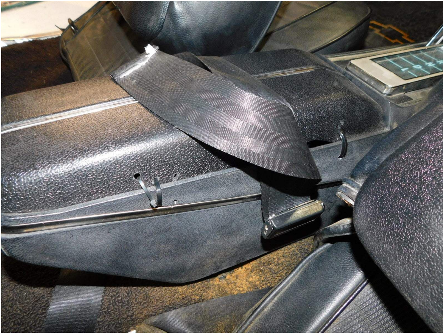
Console, damaged-zip ties used
