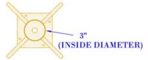
BOTTOM VIEW-POST MOUNT (NTS-BRACKET ONLY)
